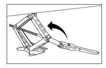
12. Lower the vehicle by turning the jack handle counterclockwise. Lower the jack completely.
